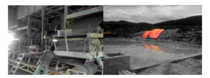
Fig. 12: Fly ash after unbured carbon separation in Pha Lai thermalpower plant
