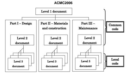
Fig. 9: Multi-level Document Structure of Asian Concrete Model Code
