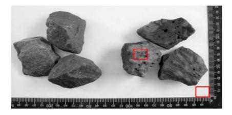
Fig. 11: Solid basalt and hollow basalt in stone mine C - Dong Nai 3
