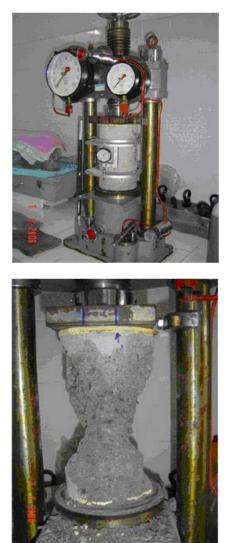
Fig.17: Experiment to determine modulus of elasticity and compressive strength of RCC
