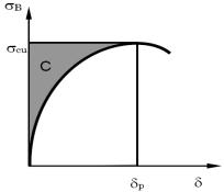
Fig. 3 The  $\sigma\text{--}\delta$  curve and the concept of complementary energy
