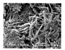
Fig. 4 Ettringite Formation of Shrinkage Compensating Concrete
