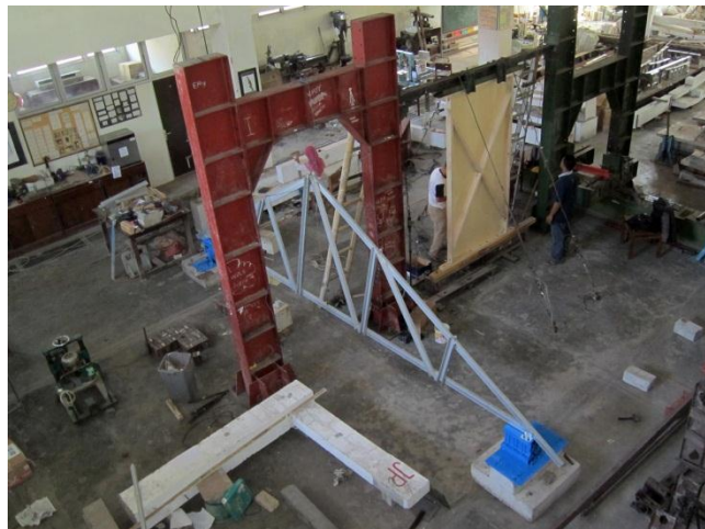
Structural Engineering Laboratory of Gadjah Mada University where test preparation of an RC beam-column joint, light steel truss and timber panel is being conducted.
