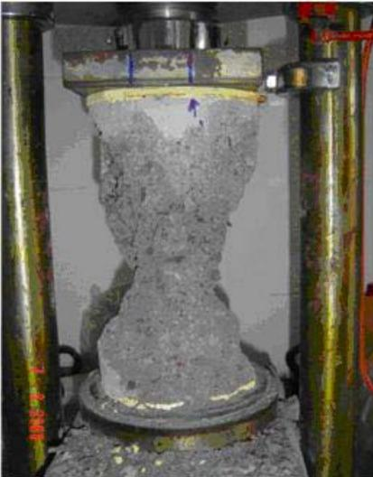
Fig.17: Experiment to determine modulus of elasticity and compressive strength of RCC
