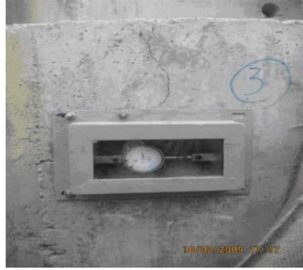
Fig. 18: RCC Cracking after construction 2 months
