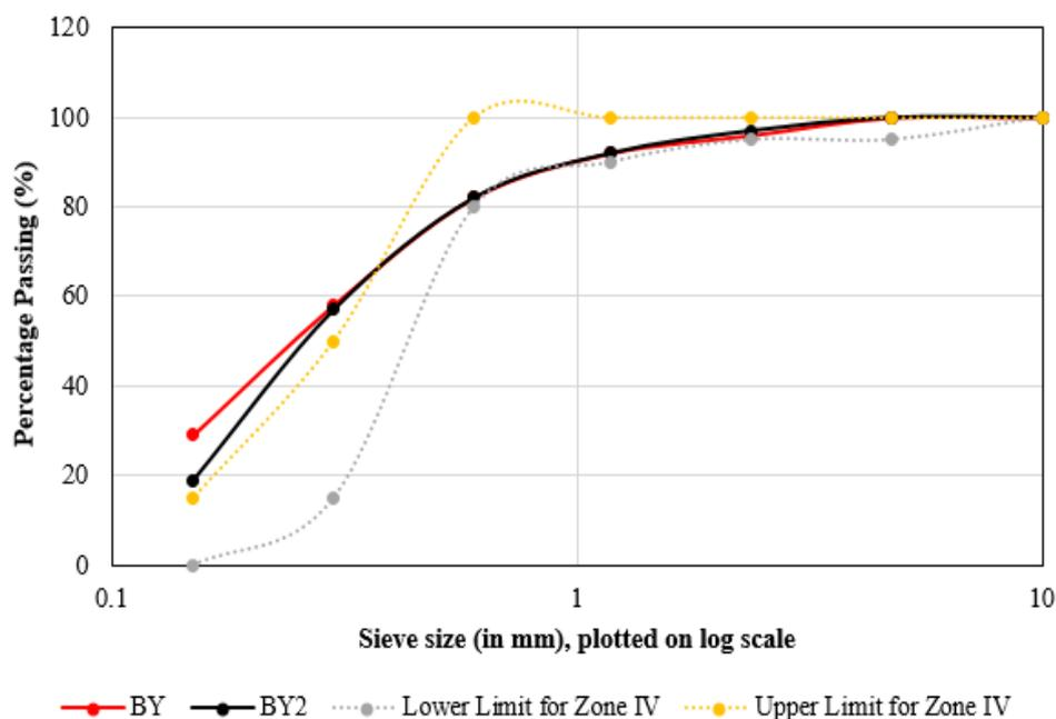
Fig. 1 – Gradation curve for sieve analysis of bottom ash BY and BY2
