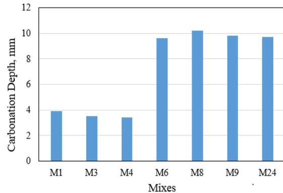
Fig. 10 – Comparison of carbonation depth results for selected mixes
