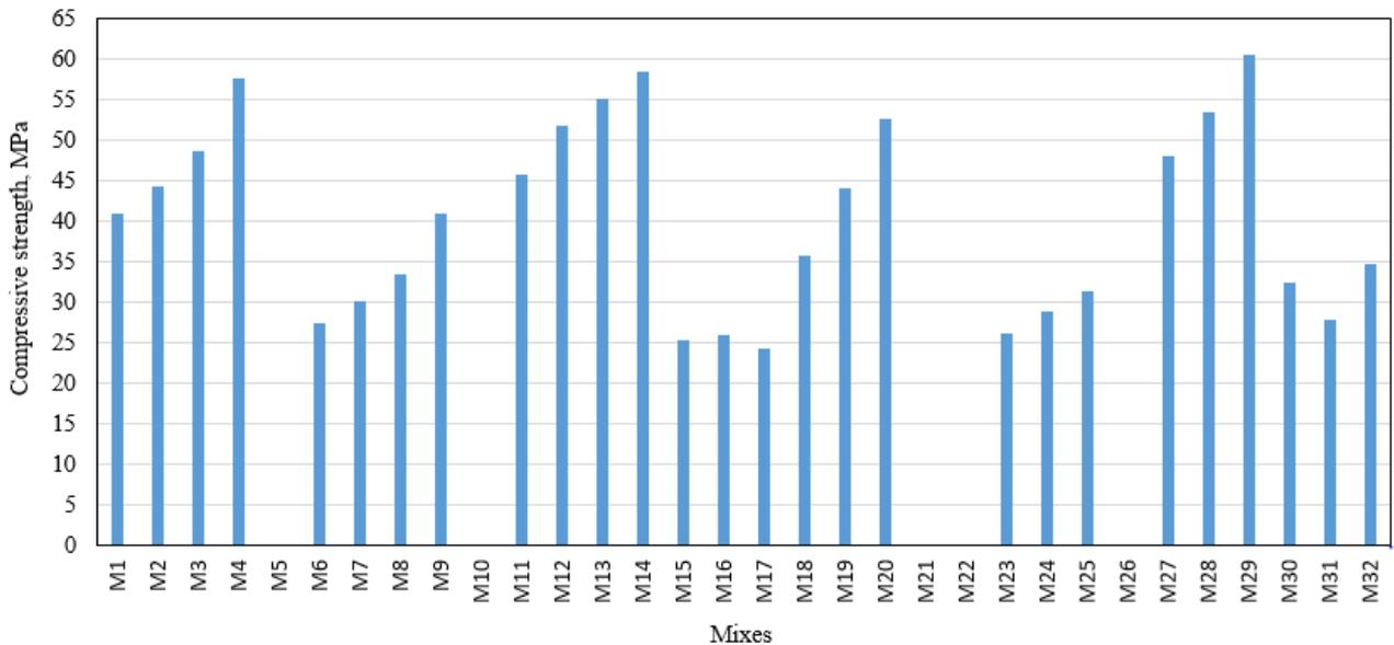
Fig. 6 – Comparison of 28-day compressive strength results for all the mixes
