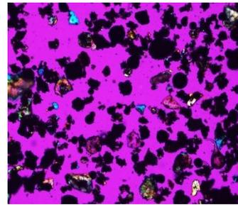
Fig. 3 – BY2- Bottom Ash (fraction between 4.75 mm and 75 μm) Distribution of mineral grains (5x)
