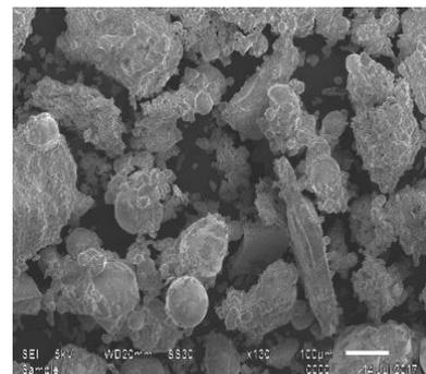
Fig. 5 – SEM image of BY2- bottom ash (fraction between 4.75 mm and 75 μm)
