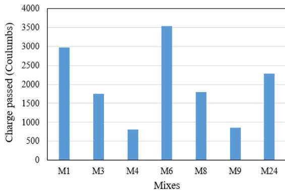
Fig. 9 – Comparison of 28-day RCPT results for selected mixes
