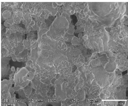
Fig. 4 – SEM image of BY- bottom ash (as such)
