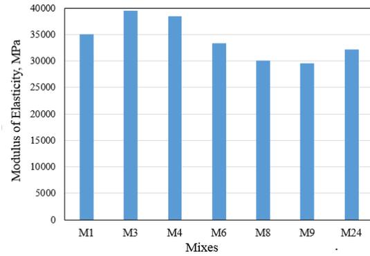
Fig. 8 – Comparison of 28-day modulus of elasticity results for selected mixes
