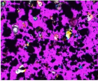
Fig. 2 – BY- Bottom Ash (As such) distribution of mineral grains (5x)
