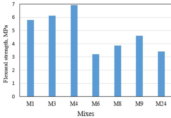
Fig. 7 – Comparison of 28-day flexural strength results for selected mixes
