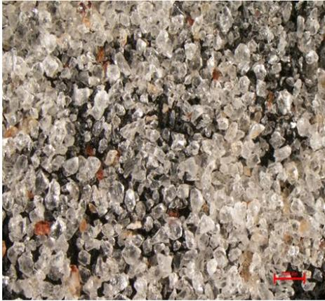
Fig 3: Distribution of minerals grains in fine Quartz sand (11.25x)
