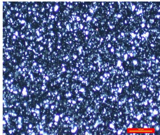
Fig 2: Distribution of minerals grains in Ground Quartz. (5x, X-Nicols)
