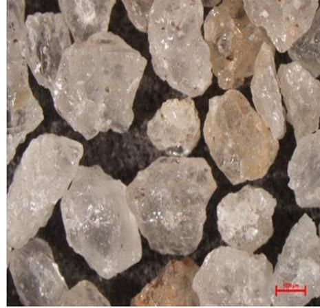
Fig 4: Distribution of mineral grains in Coarse Quartz sand sample (11.25x)
