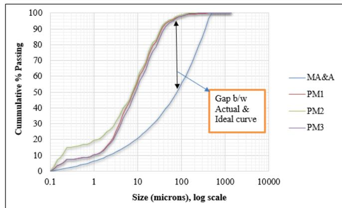
Fig 6: Grading of ideal curve and designed mixes
