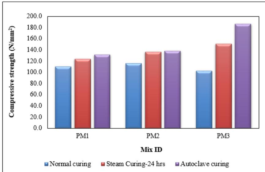
Fig 7 Compressive strength for three different curing regimes
