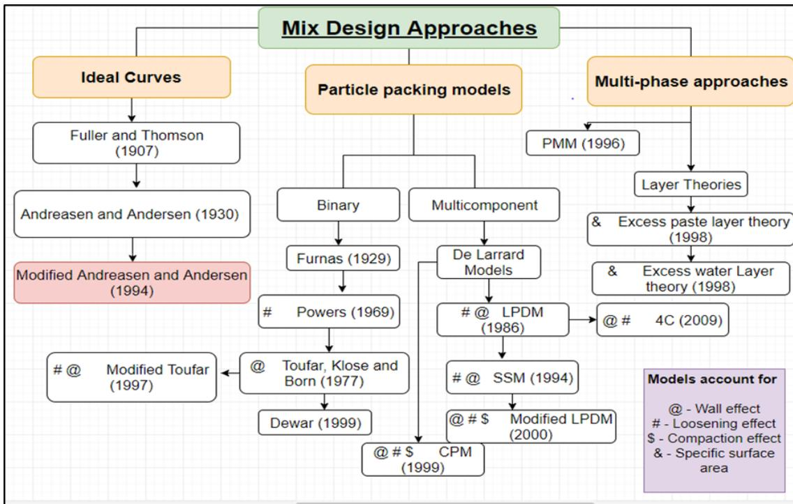
Fig 1: Mix design approaches for optimizing packing density [13]
