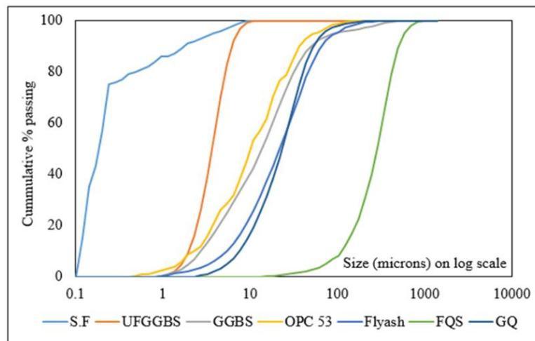
Fig 5: Particle size distribution of materials
