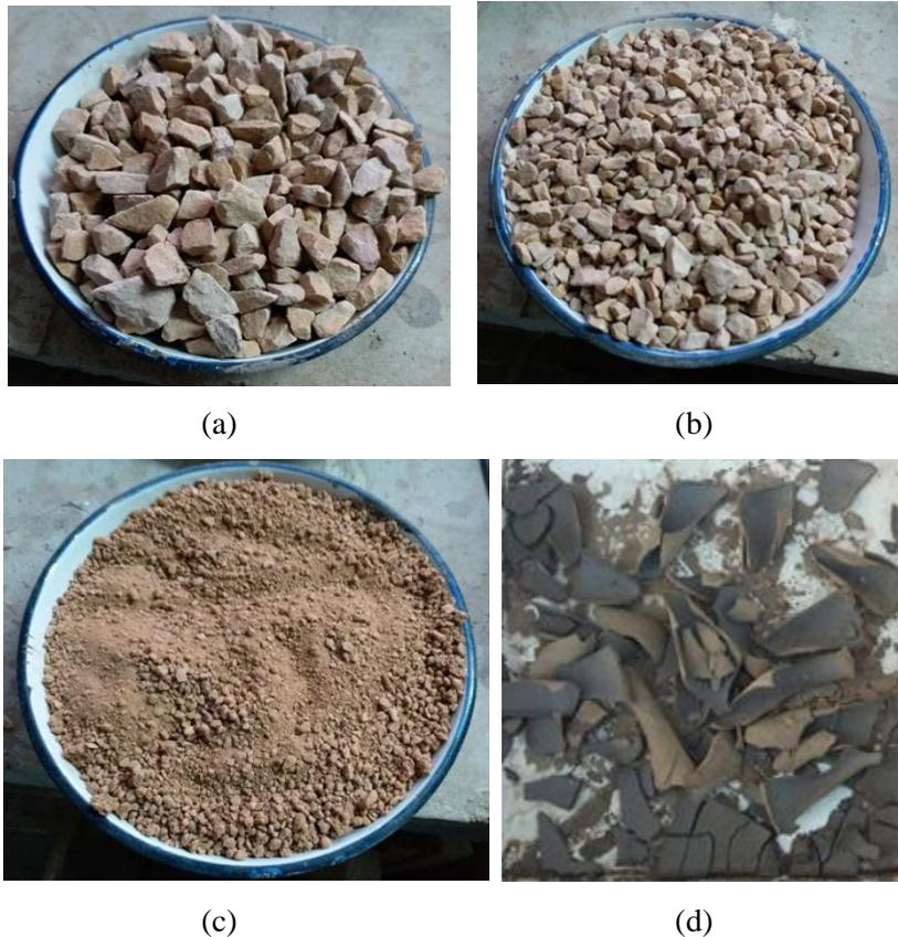
Fig 2: Aggregates (a) 20 mm; (b) 10 mm; (c) crushed sand; (d) deleterious material: prepared clay before being pulverized
