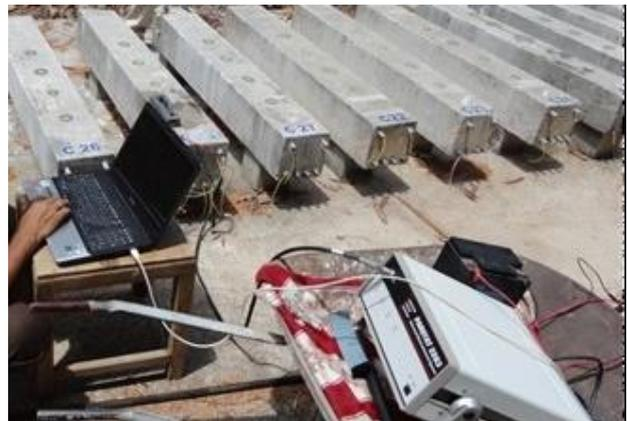
Fig. 2 – EIS measurement on PS beam is in progress
