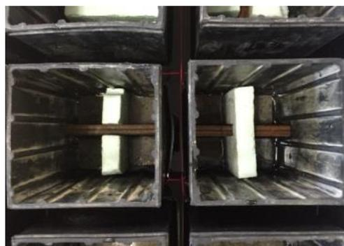
Fig. 1 – Mortar specimens in the sleeve
