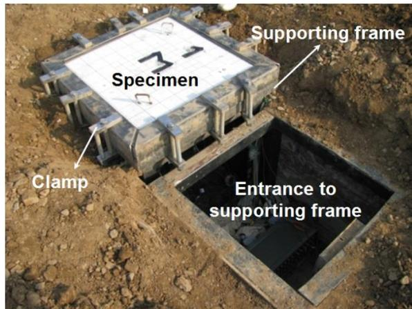
Fig. 3 – Configuration photo of buried supporting frame
