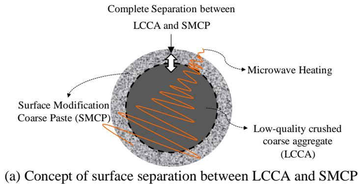
(a) Concept of surface separation between LCCA and SMCP
