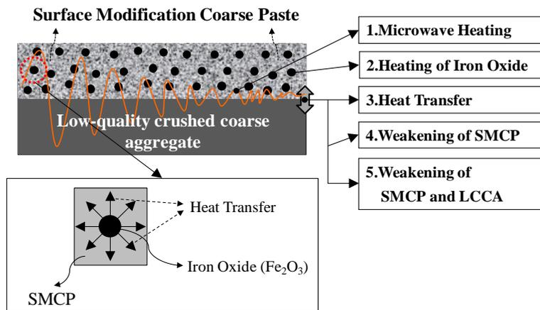
(b) Control factor of surface separation of modification aggregate
