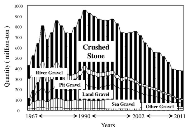
Fig. 1 – Changes in the aggregate supply in Japan [1]
