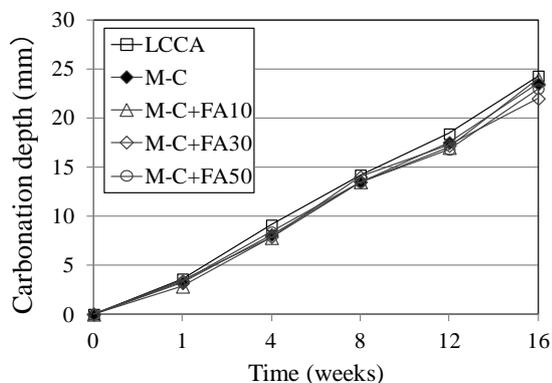
Fig. 8 – Carbonation depth
