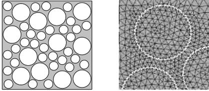
Fig. 1 FEA for Strength Based Gradation of High Strength Concrete
