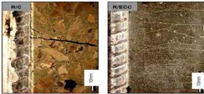
Fig. 5 Compatible deformation between ECC and steel reinforcement (right)
