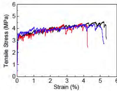
Fig. 2 Uniaxial tensile stress-strain curves of an ECC reinforced with 2% PVA-REC15 fibers
