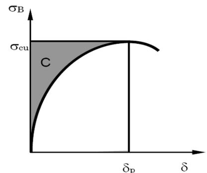
Fig. 3 The  $\sigma$ - $\delta$  curve and the concept of complementary energy
