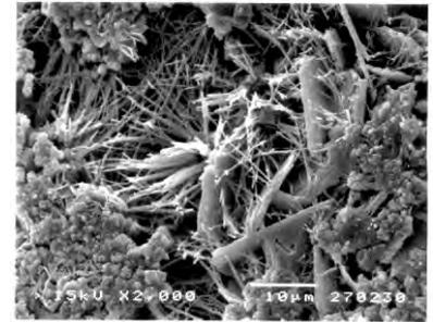
Fig. 4 Ettringite Formation of Shrinkage Compensating Concrete
